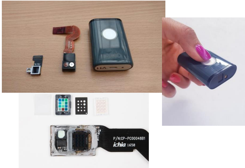
Figure 1. The SCiO spectral sensor and some details of the inside components including source, detector, filters with mask for signal equalization, and a microlens array for optimized light coupling to detector.
